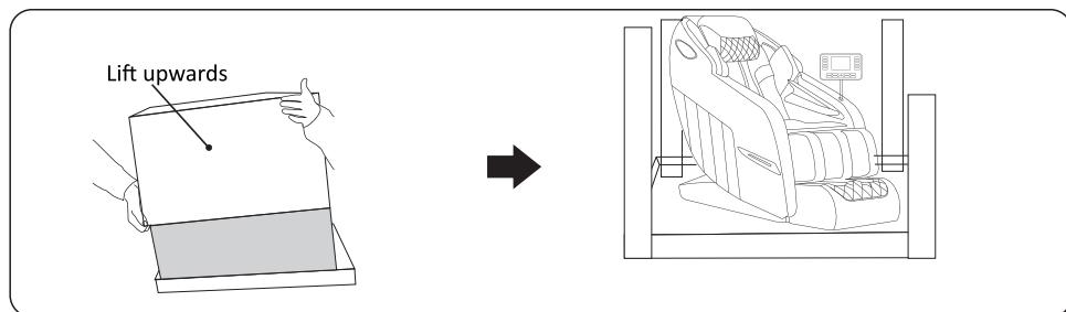
1) Cut off the packing strap and lift up and move away the carton.
